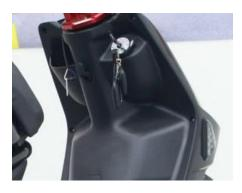
Turn power switch to 'ON' position : the motor can be started.
